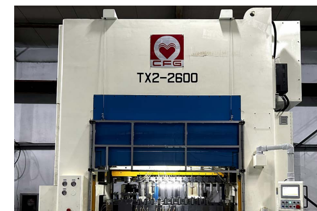
260 Ton 2 Point for EV Battery Shell
